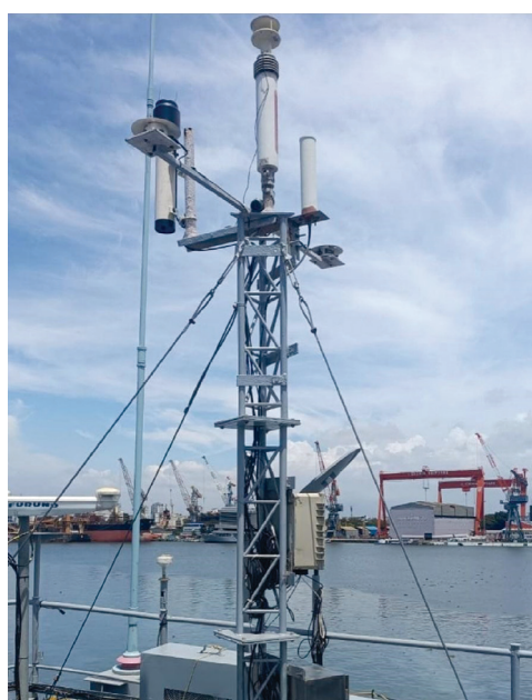
Figure 6.8 (left) The newly installed AWS onboard INS Investigator. (right) AWS data availability.
